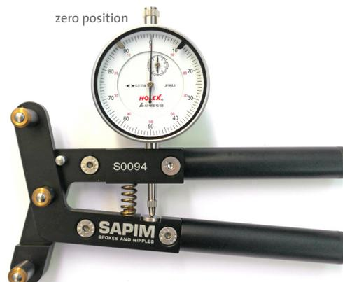
Press the handles together and put the tensiometer on the spoke so that the spoke lays between the bearings (see picture).
