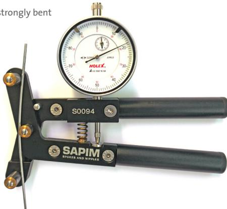
High spoke tension - high reading
