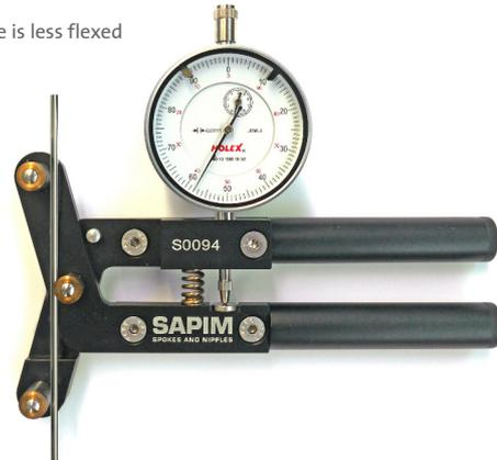
The tensile force of the spoke is indirectly measured by the deformation of the spoke.
